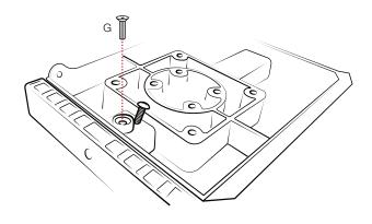
2 Using a screwdriver, press springs into tray. While holding springs down, wedge one of the (E) screws into the smaller hole to jam the springs in place. Remove pen or screwdriver.
